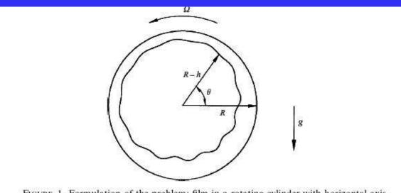
FIGURE 1. Formulation of the problem: film in a rotating cylinder with horizontal axis.
