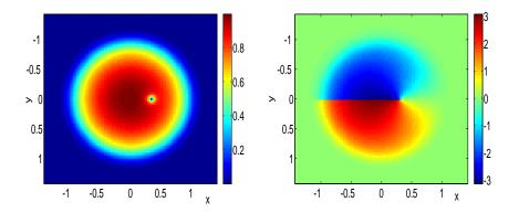
Spatial contour plots of the amplitude (left) and phase (right) of a rotating charge-one vortex.
