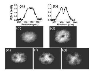
Absorption images of a BEC stirred with a laser beam. From Madison et al., 2000.
