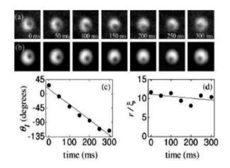
Vortex precession in a trapped two-component BEC. From Anderson et al., 2000.
